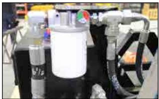
Fig 70 - Hydraulic oil filter
