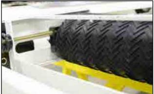
Fig 38 - Six Inch tail roller
