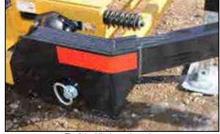
Fig 24 - Hitch anchor pins
