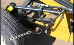
Fig 26 - Axle locking pin
