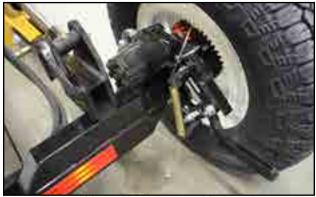
Fig 23 - Mover kit drive assembly - version 2
