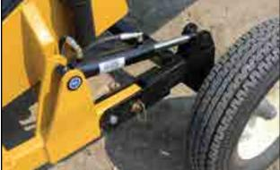
Fig 53 - wheel axle lift cylinders
