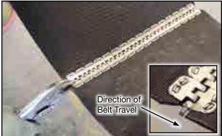
Fig 59 - Crimp lacing and tapered corners
