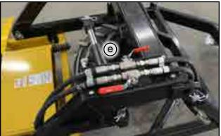
Fig 21 - Ball valves for transport
