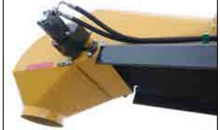
Fig 45 - Discharge spout with hydraulic drive
