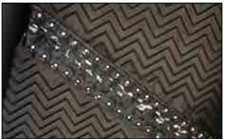
Fig 39 - Super screw® lacing
