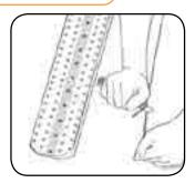
Chamfer the end of the belt top and bottom as shown. Position Super-Screw<sup>®</sup> against the belt, ensuring that Super-Screw® is resting against the central spacers.
