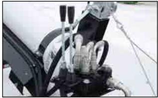
Fig 13 - Hydraulic valves
