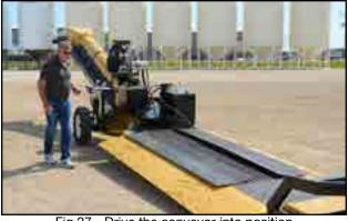
Fig 27 - Drive the conveyor into position
