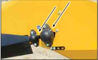
Fig 52 - Discharge roller bearings grease zerks
