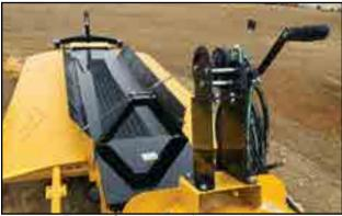
Fig 17 - Containment flaps and winch
