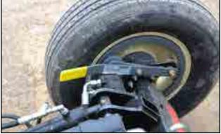
Fig 25 - Disengage drive wheel handle
