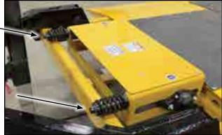
Fig 56 - Tail roller tension bolt
