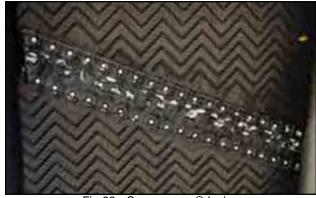
Fig 62 - Super-screw® lacing
