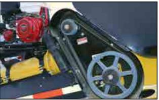
Fig 65 - Countershaft to belt roller belt
