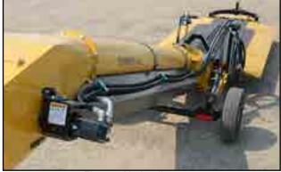
Fig 12 - Hydraulic motor
