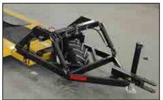
Fig 54 - Self-propelled mover kit steering wheel
