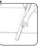
Cut your belt with a 1/3 bias (or 10% min of the width of the belt). The other side of the belt should be cut with a bias in the opposite direction.
