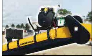
Fig 8 - Gas engine mounted on tube
