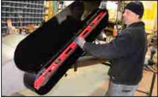
Fig 69 - Pulley alignment
