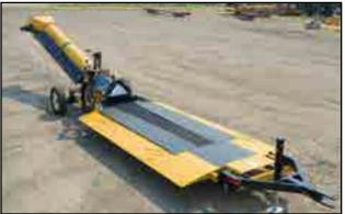
Fig 41 - Conveyor being stored
